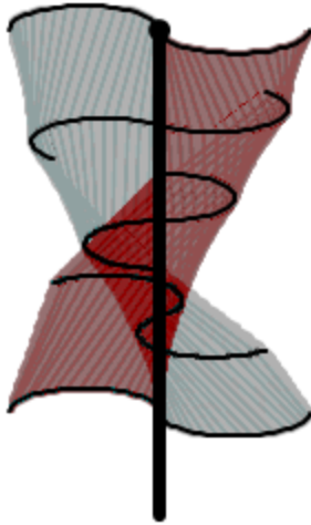
Figure 4: A vertical axis Twisted Savonius type turbine.
