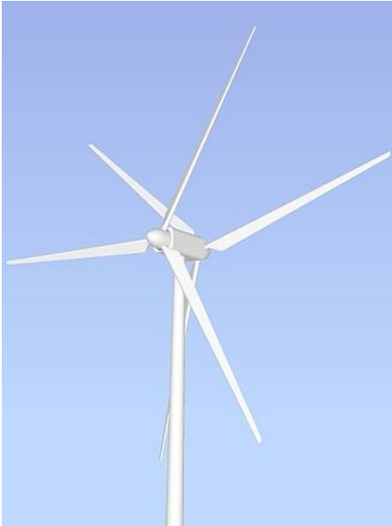
Figure 9: Counter rotating wind turbine (dual rotor)
